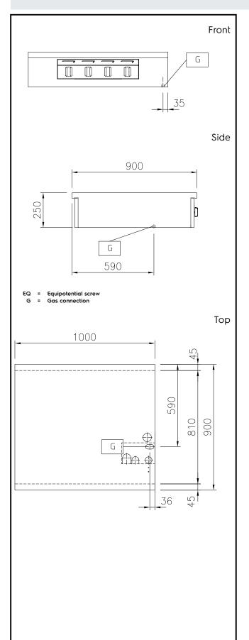
Gas Gas Power: 40 kW Gas Type Option: Gas Inlet: 1/2" **Key Information:** External dimensions, Width: 1000 mm 900 mm External dimensions, Depth: External dimensions, Height: 250 mm Net weight: 82 kg Configuration: One-Side Operated;Top ISO 9001; ISO 14001 - ISO 9001; ISO 14001 kW Front Burners Power: **Back Burners Power:** 10 - 10 kW **Back Burners Dimension -**Ø 70 Ø 70 Front Burners Dimension -
